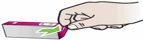
**CAUTION:** Be careful not to bend the tab out more than 1.27 cm (0.5 inches). Moving the tab too far might damage the cartridge or cause the tab to break off
