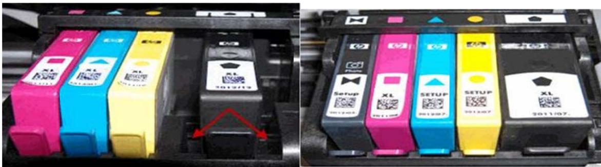
HP has put expiration dates (and new part numbers) on the 564/564XL cartridges. Stamped onto the bottom of the cartridge between the chip and the ink port is a date (and new part number)
