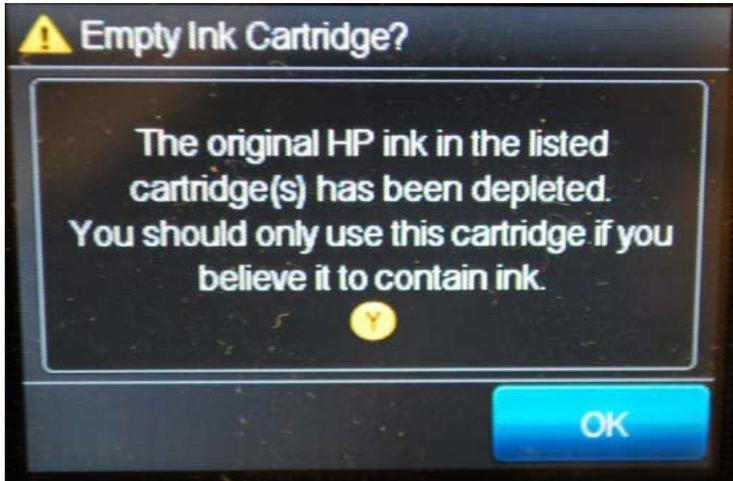
In addition, the following screen might come up when the customer uses a refilled cartridge that they have just purchased. Instruct your customer that it is ok to press yes and continue printing. We have tested multiple cartridges. When the cartridge is truly out of ink the printer will state the cartridge is empty, and will not print until another refilled cartridge is inserted
